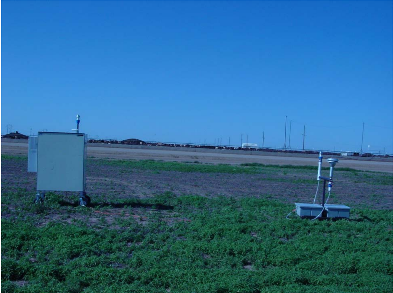
Figure 2. Co-located TSP/PM 10 samplers (right) placed with a TEOM sampler (left) at the south location at the feed yard. There is a 1 meter distance between the co-located inlet heads and approximately 10 meters between the co-located samplers and the TEOM sampler.
