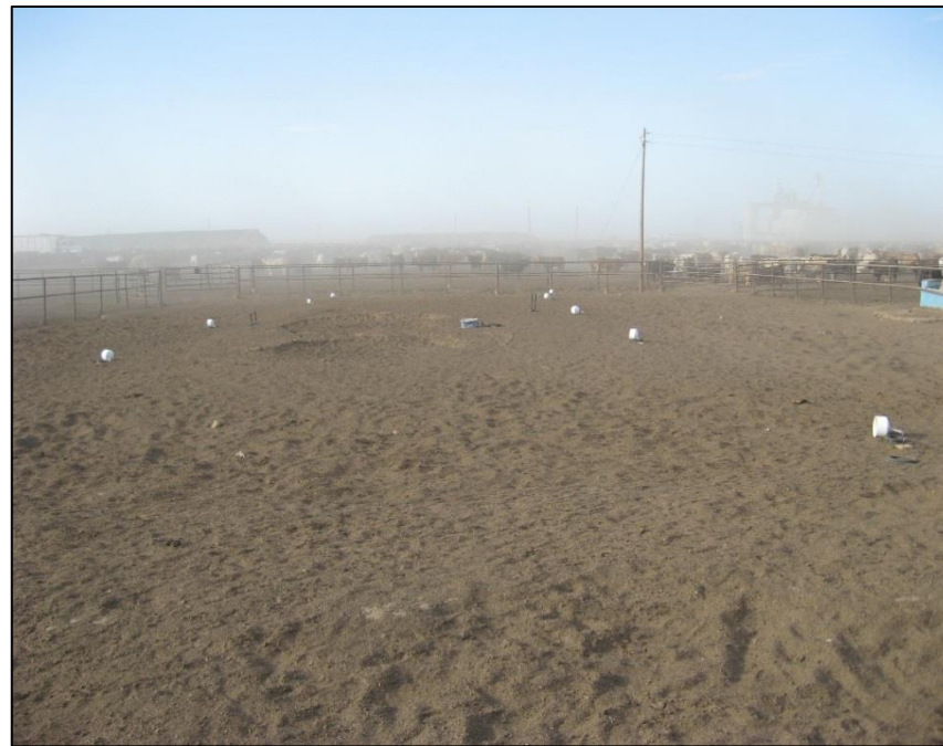
Two rows of five NFT-NSS chambers installed in a pen at Feedyard-C.
