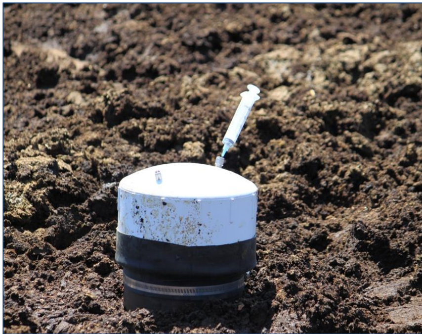
NFT-NSS chamber with top installed and sealing skirt rolled up.
