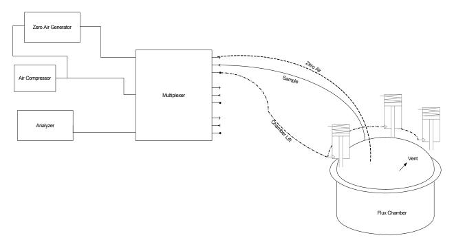
Figure 1. Multiplexed chamber setup.
