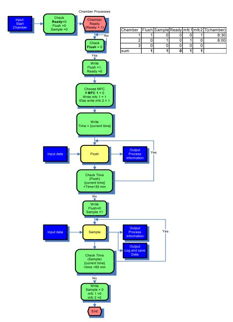
Figure 3. Multiplexer process diagram.
